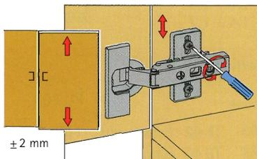
Using height-adjustable mounting plates
