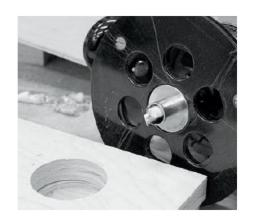
Cutouts for vertical wall applications should be made oversized by at least 1/8" all around to allow for expansion and contraction. Radius all inside corners with a minimum 1/4" radius and sand all edges smooth.
